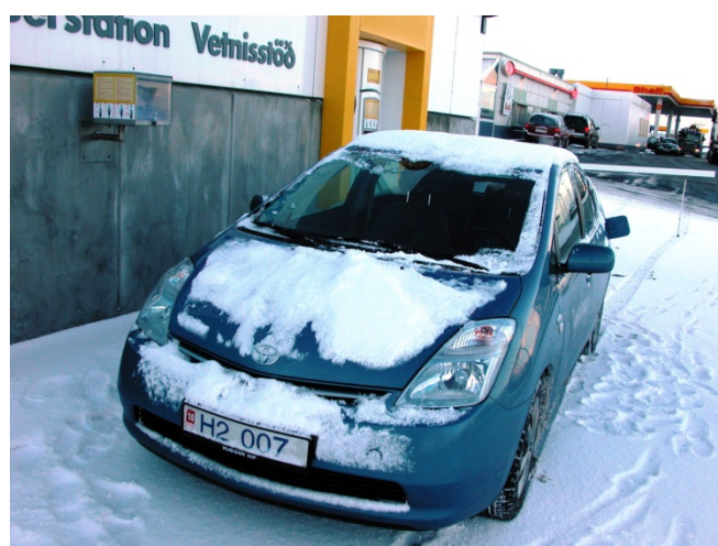
During the coldest spell of the winter some performance difficulties arose in the Prius' cars, but after installing plug-in engine and space heaters the cars have been performing very well.
